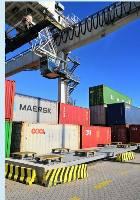
Installation of the Container Weighing System in METRANS Prague, Czech Rep.
