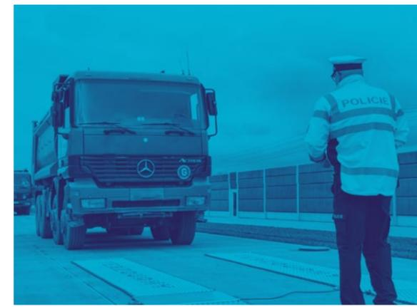
The mobile wheel and axle weighing system is designed for weighing road cargo vehicles, their wheels and axles. The capacity of this weighing system is not limited either by the length of the vehicle combination or its total weight, only the weight of each axle must be less than 20 tons, which is sufficient by a large margin for weighing road vehicles and vehicle combinations on the road.
