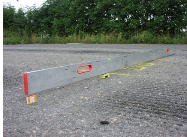
The longitudinal unevenness is greater than the permitted 2% and thus more than 2 cm / 1 m
