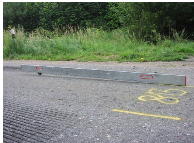
The transverse unevenness is greater than the permitted 2% and thus more than 2 cm / 1 m
