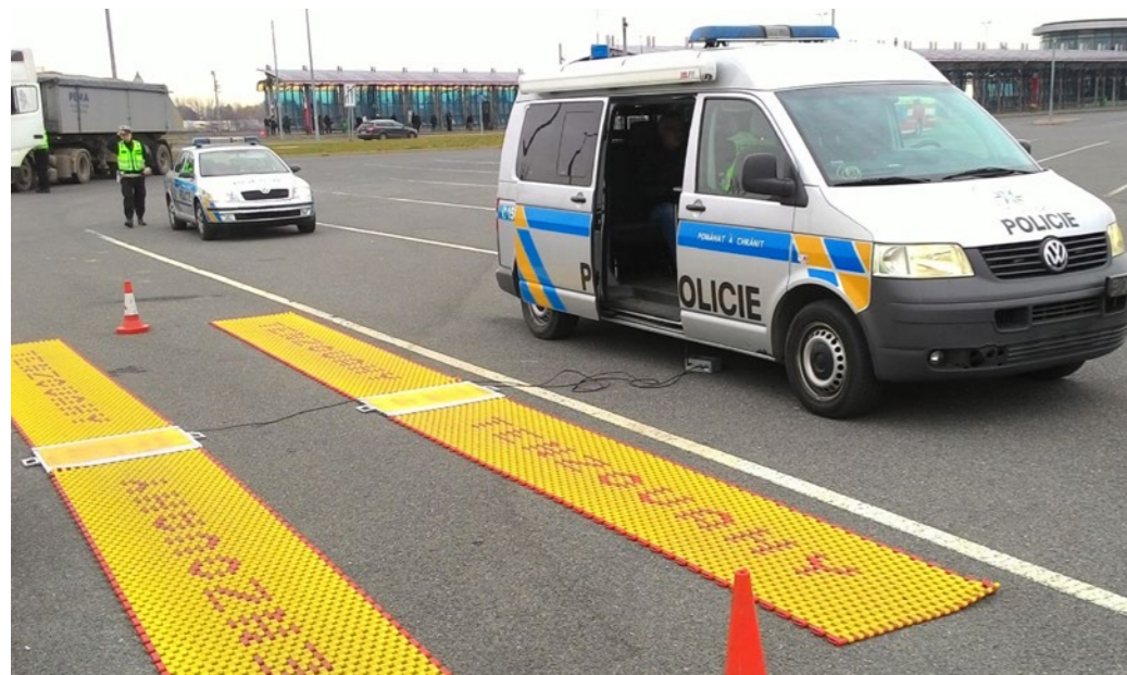
Use of Portable Scales PW-10 by members of the Police of the Czech Republic
