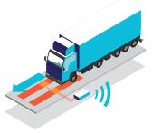
The thin and light weighing device PW-10 combines reliability with high mobility in everyday operation. The system is ready for weighing within minutes. The weighed vehicle is continuously guided by a weighing zone consisting of a pair of weighing pads and four rolling mats.
