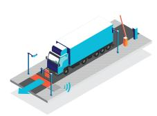
The Axle Scales TENZOWIM 134 determines total vehicle weight, loading of axles and groups of axles, i.e. weight parameters that cannot be determined by usual static scales. Thanks to the high throughput of the scales, no congestions are formed at the entrances or exits to/from facilities, which greatly speeds up the whole process of dispatching vehicles.
