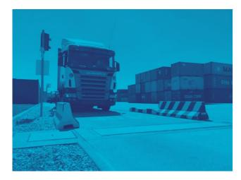
The TENZOWIM 134 Axle Weighing System is used for automatic weighing of road vehicles driving at lower speeds (about up to 30 km/h) without the need to stop. This is a dynamic weighing system. It is distinguished by low operating costs and high accuracy. Its use is in weighing for law enforcement by state authorities and in many sectors of industry.
